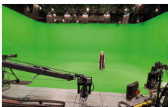
The studio's VR set is 130 square meters and uses three tripod mounted URSA Broadcasts as well as a dolly mounted 4.5m jib on a six meter track. An ATEM 4 M/E Broadcast Studio 4k, with ATEM 1 M/E Advanced Panel, is used for live vision mixing.
